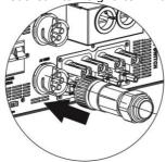
**CAUTION:** To prevent risk of electric shock, ensure the ground wire is properly earthed before operating this hybrid inverter no matter the grid is connected or not.
