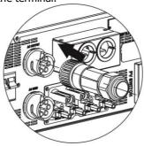
**CAUTION:** It's only allowed to connect load to "AC Output Connector". Do NOT connect the utility to "AC Output Connector".
