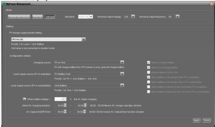
PV energy supply priority setting: 1<sup>st</sup> Load, 2<sup>nd</sup> Battery
