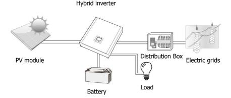
Figure 1 Basic hybrid PV System Overview
