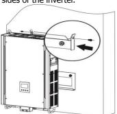
2. Raise the inverter and place it over the mounting plate.
