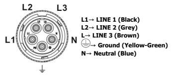
The reference tightening torque is 1.5-2.5 N.m.
