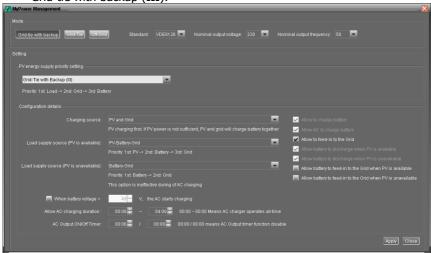
PV energy supply priority setting: 1<sup>st</sup> Load, 2<sup>nd</sup> Grid and 3<sup>rd</sup> Battery
