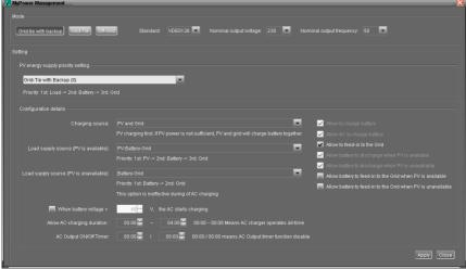
PV energy supply priority setting: 1st Load, 2nd Battery and 3rd Grid.
